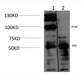
Western blot analysis of 1)MCF7 Cell, 2) Mouse Brain Tissue Lysate using NF kB P105/P50Mouse Monoclonal mAb diluted at 1:1,000.
